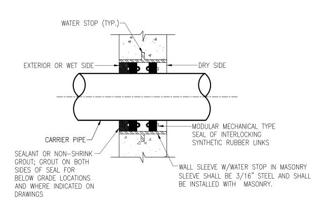
1. CONCRETE SHALL BE WORKED IN AND VIBRATED TO ELIMINATE ALL VOIDS IN CONCRETE. IF VOIDS DO REMAIN, FILL WITH GROUT BEFORE INSTALLING PIPE AND
