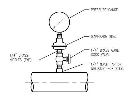
PROVIDE SNUBBER FOR ALL INSTALLATIONS. PROVIDE DIAPHRAGM SEALS FOR ALL WASTEWATER SERVICES OTHER THAN SLUDGE. LOCATE PRESSURE TAPS ON TOP OF PROCESS PIPING. . FOR STEEL, VAL. STEEL, AND PVC 2.5" AND SMALLER USE A BUSHING IN A TEE. . FOR DI AND FRP PIPE, ALL SIEZES, USE PIPE SADDLE WITH BUSHING. 6. FOR STEEL AND SS PIPES 3" AND LARGER, AND PRESSURE VESSELS, USE THRED-O-LET.
