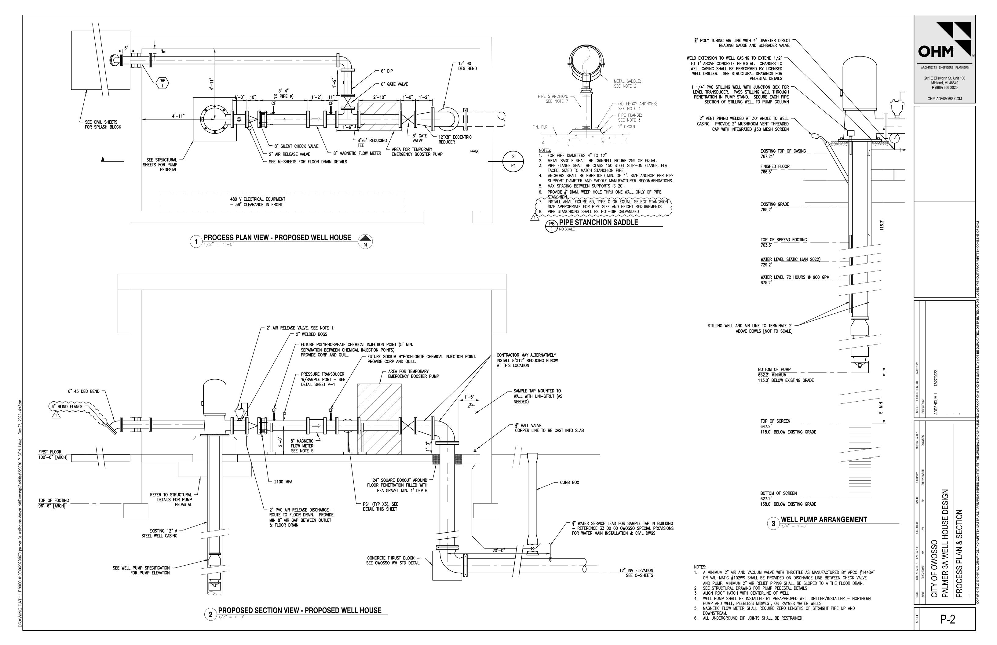
2. EXTERIOR PIPING IS SHOWN ON THE CIVIL DRAWINGS. 3. DIELECTRIC COUPLINGS, FLANGES OR UNIONS SHALL BE INSTALLED AT ALL CONNECTIONS OF
